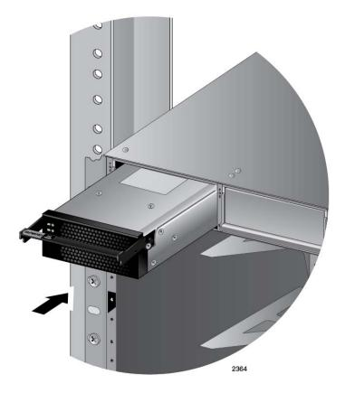
Figure 60. Inserting the AT-SBxPWRPOE1 AC Power Supply
